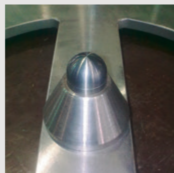
Hardened, nearly maintenance free bottom pintle bearing.
