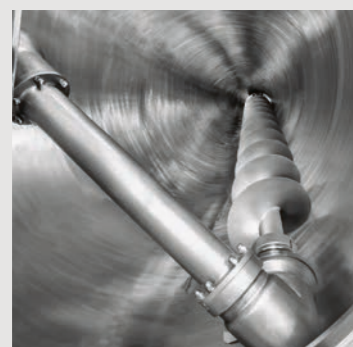
Arm for orbital movement and agitator screw for vertical movement
